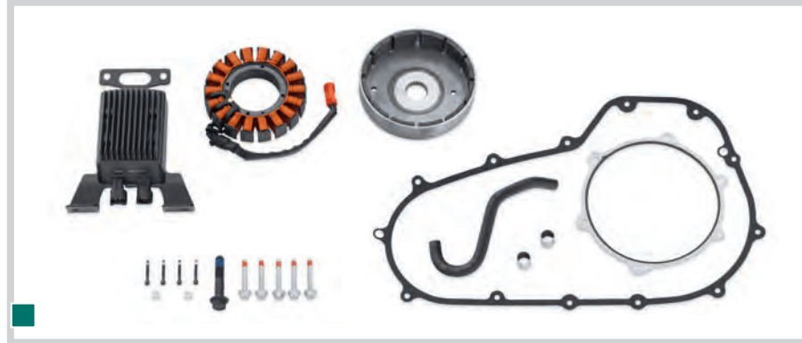
C. 54-AMP HIGH OUTPUT CHARGING SYSTEM
