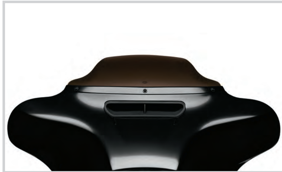
C. 7" WIND SPLITTER ST WINDSHIELD - BATWING FAIRING
